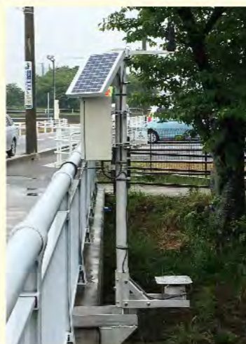
Installation example of ultrasonic wave gauge
